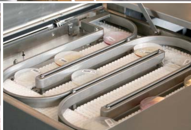
Above: This is how the PK dilution plating machine is currently operating in Spijkenisse. Left: All pipette operations in Spijkenisse are fully LIMS-guided. Right: Snaking design with cooling conveyor belt saves lots of space in SGS Spijkenisse.
