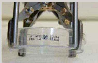
Gripping device designed for SGS Portugal, lifts cover in order to print 2D code high up the side.
